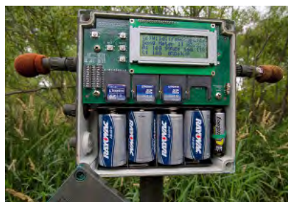
Researchers use this device to record sound for five minutes every hour — night and day.
