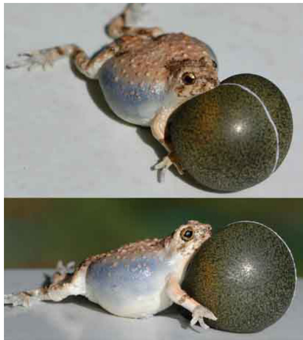
Barrett Klein’s robotic frogs. The faux frogs, with pneumatically-controlled vocal sacs made of catheters.
