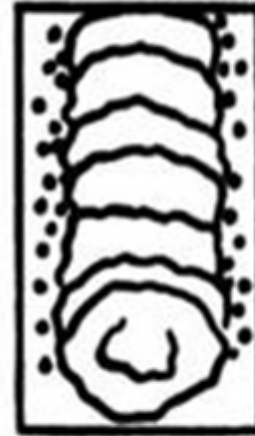
Welding current too high
