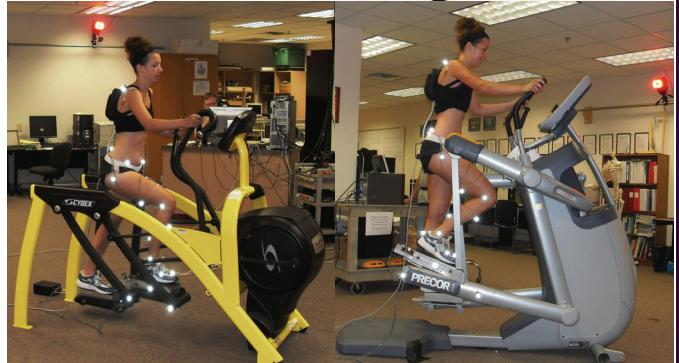
Two elliptical machines being evaluated by LIMS researchers. Reflective markers allow cameras to measure movement by cameras. A pedal is instrumented with a force platform
