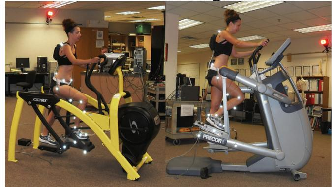
Two elliptical machines being evaluated by LIMS researchers. Reflective markers allow cameras to measure movement by cameras. A pedal is instrumented with a force platform
