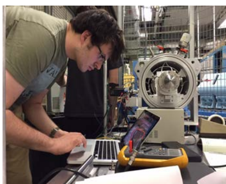
Graduate Student Jack Dermigny programming the movable extraction electrode for the new LENA ECR source.
