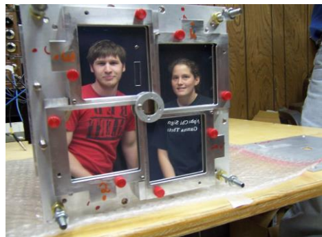
Detector used for four-body decay measurements. This small detector array is part of the larger HiRA array built in collaboration with MSU and IU. Images of two former students can be seen reflecting off the Si detectors.
