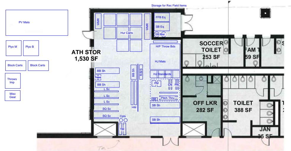
Floor Plan - Level 1, Storage Detail (North End, West)
