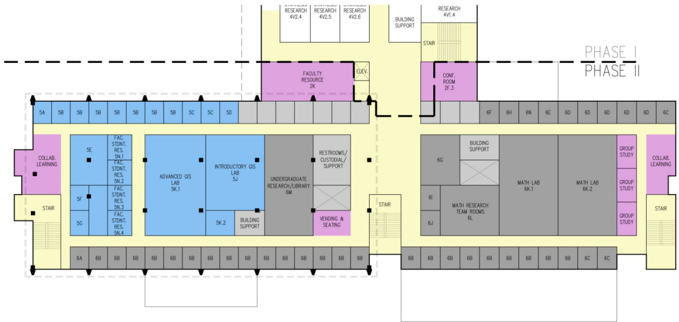
Third Floor Plan/Phase 2 Renovation + New Addition Option
