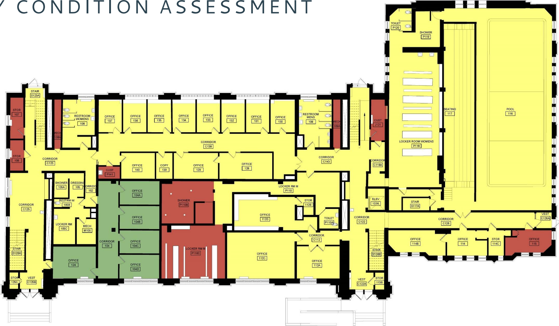
NORTH 1 GROUND LEVEL - CONDITION 1/8" = 1'-0"
