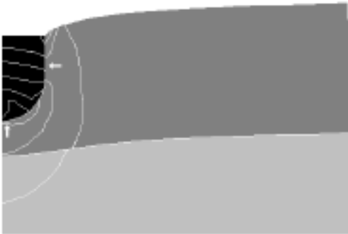
Figure 3 Contour plot of 3rd principal stress for a 16 cm cushion. The arrows indicate the areas of highest compressive (bottom arrow) and shear (top arrow) stress.
