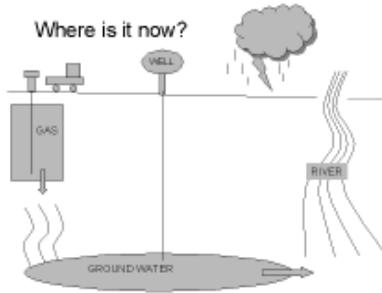
FIG. 1. MTBE leaking from gas station storage tanks infiltrates ground water supplies which eventually interact with surface waters. Once in surface waters, evaporation allows MTBE to travel through the atmosphere associated with various forms of precipitation. The most dangerous consequence of groundwater contamination is poisoning of fresh water supplies.
