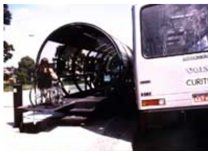
Figure 5. Handicap accessibility of Bus Tubes
