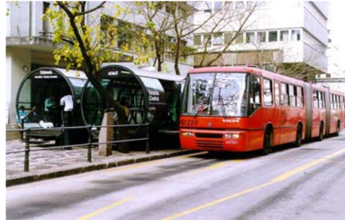
Figure 2. Photo of Bus Tubes and Bi-Articulated Bus in Curitiba
