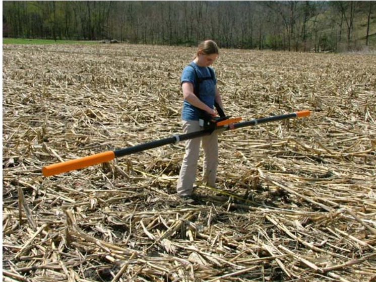
Figure 3. Taking conductivity measurements
