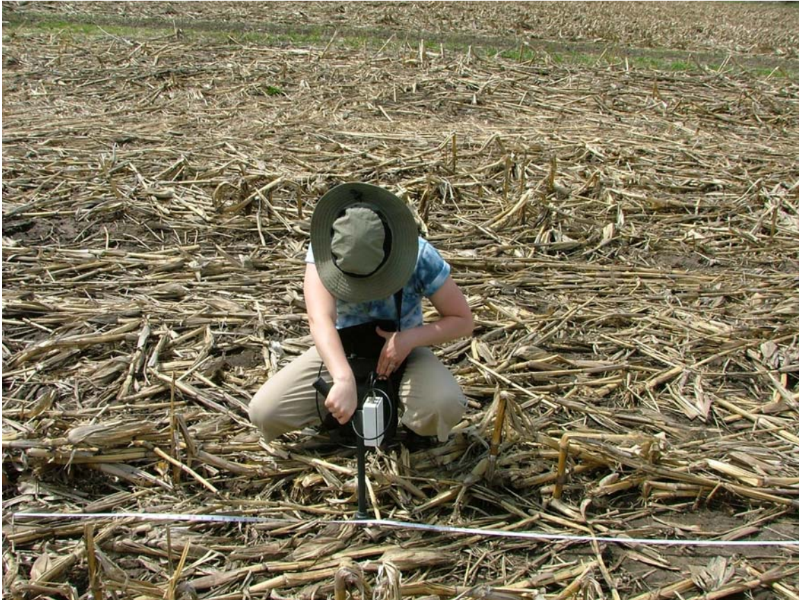
Figure 9. Taking surface measurements with the MS2F probe
