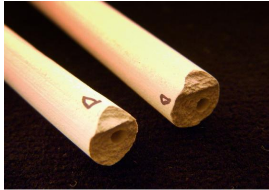
Plate 19. Common Flaking Pattern to the Accidentally Broken Fragments
