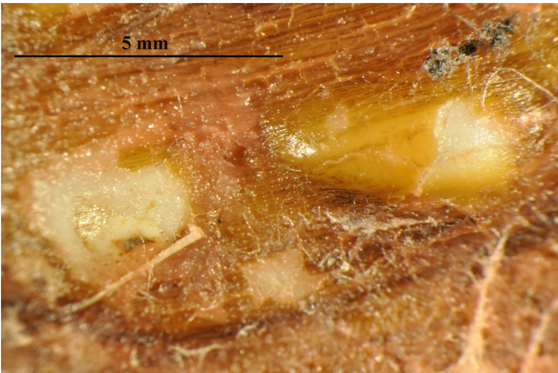
Figure 30. Close up of pustule wear on right valve of pimpleback experimental applicator (26x)
