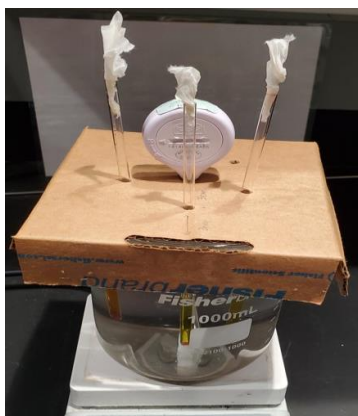
Figure 3. Illustration of setups used for tested curcuminoid: A. water bath, B. samples under UV-A light in the instrument's chamber.
